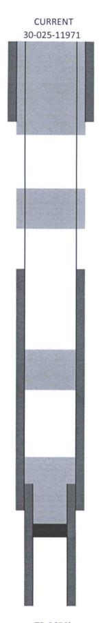
CUT OFF WELLHEAD, VERIFY CEMENT TO SURFACE, & INSTALL BELOW GROUND DRY HOLE MARKER (LPC AREA)
