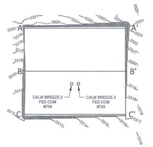
Top of pad elevation: 3317.1609 Cut Slope: 33.33% 3.00:1 18.43° Fill Slope: 33.33% 3.00:1 18.43° Balance Tolerance (C.Y.): 0.00 Cut Swell Factor 1 00 Fill Shrink Factor, 1.00
