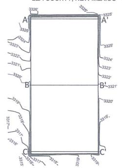
Top of pad elevation: 3321.2690 Cut Slope: 33.33% 3.00:1 18.43° Fill Slope: 33.33% 3.00:1 18.43° Balance Tolerance (C.Y.): 0.00 Cut Swell Factor: 1.00 Fill Shrink Factor: 1.00
