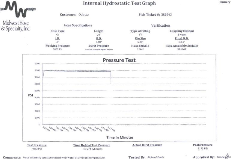
Comments: Hose assembly pressure tested with water at ambient temperature.
