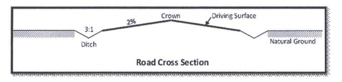
f. The access road will be constructed with a ditch on each side of the road.
