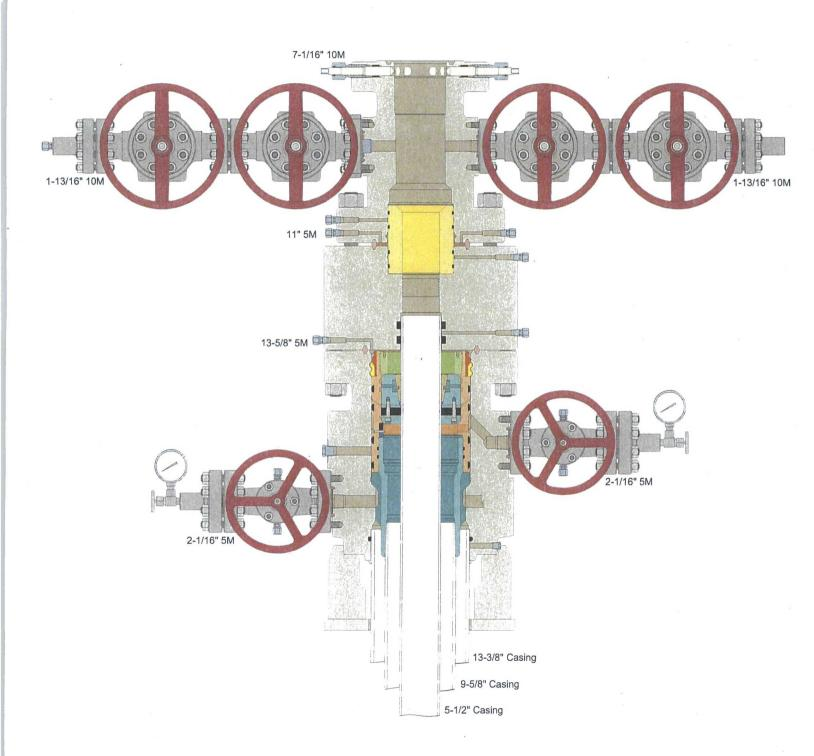
A multibowl wellhead may be used. The BOP will be tested per Onshore Order #2 after installation on the surface casing which will cover testing requirements for a maximum of 30 days. If any seal subject to test pressure is broken the system must be tested.
