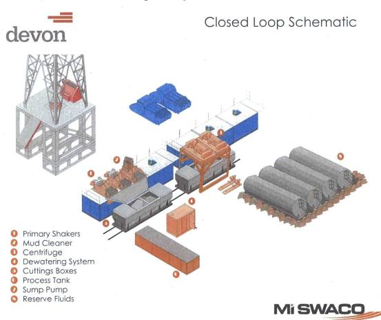
Centrifuges: The centrifuges can be one or two in number depending on the well geometry or depth of well. The centrifuges are sized to maintain low gravity solids at 5% or below. They may or may not need a dewatering system to enhance the removal rates. The centrifuges can make a cut point of 8-10 microns depending on bowl speed, feed rate, solids loading and other factors.
