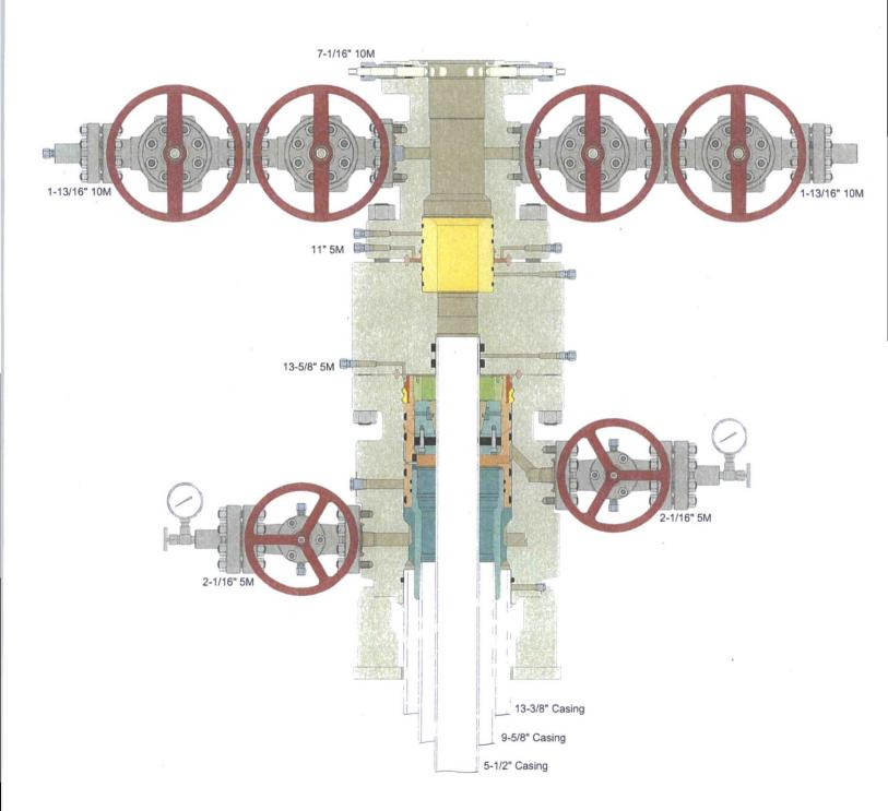
A multibowl wellhead may be used. The BOP will be tested per Onshore Order #2 after installation on the surface casing which will cover testing requirements for a maximum of 30 days. If any seal subject to test pressure is broken the system must be tested.
