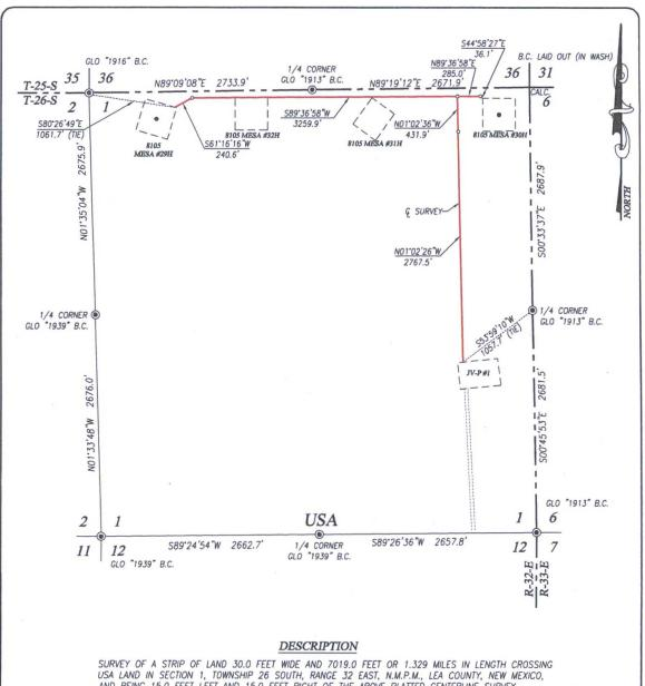
SURVEY OF A STRIP OF LAND 30.0 FEET WIDE AND 7019.0 FEET OR 1.329 MILES IN LENGTH CROSSING USA LAND IN SECTION 1, TOWNSHIP 26 SOUTH, RANGE 32 EAST, N.M.P.M., LEA COUNTY, NEW MEXICO, AND BEING 15.0 FEET LEFT AND 15.0 FEET RIGHT OF THE ABOVE PLATTED CENTERLINE SURVEY.
