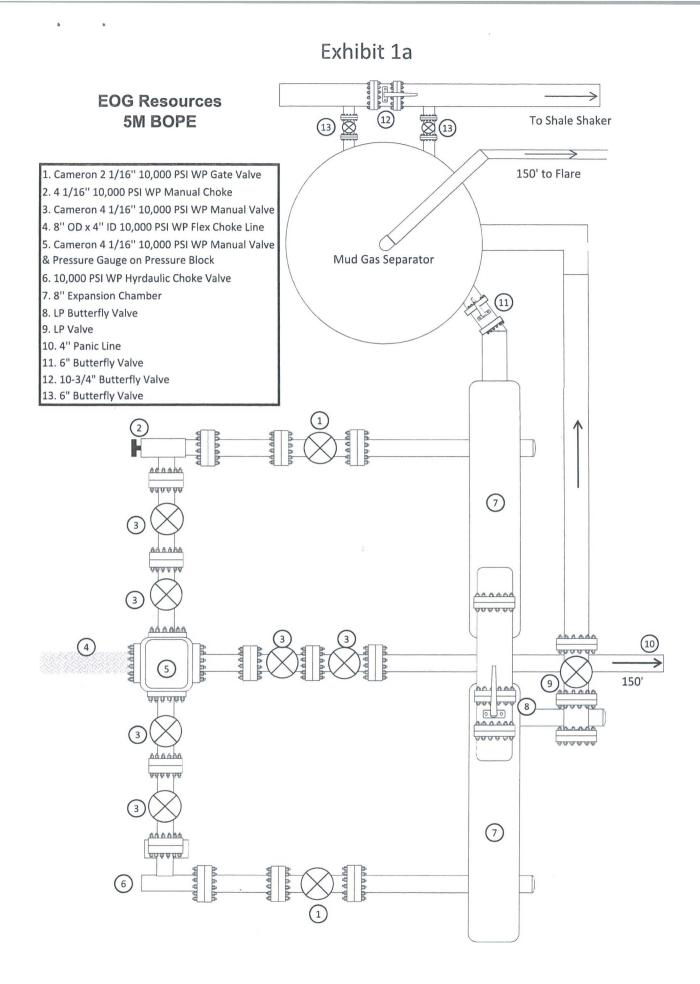
EOG 5M Choke Manifold Diagram (rev. 3/21/14)
