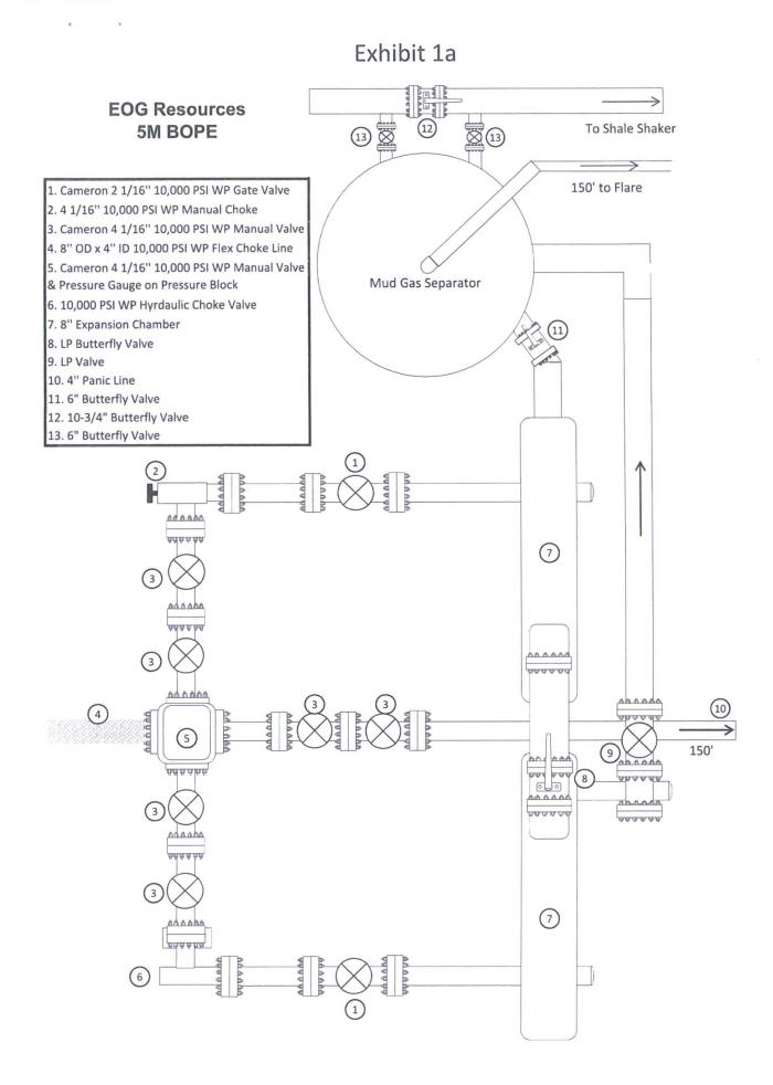
EOG 5M Choke Manifold Diagram (rev. 3/21/14)
