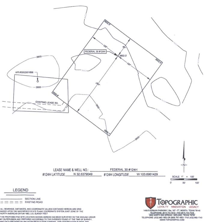
ALL BEARINGS, DISTANCES, AND COORDINATE VALUES CONTAINED HEREON ARE GRID BASED UPON THE NEW MEXICO STATE PLANE COORDINATE SYSTEM, EAST ZONE OF THE NORTH AMERICAN DATUM 1983, U.S. SURVEY FEET
