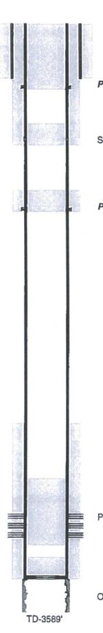
13" hole @ 390' 10-3/4" csg @ 387' w/ 250sx-TOC-Surf-Circ
