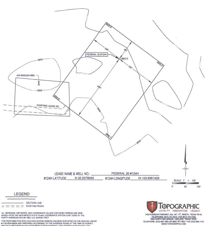
NORTH AMERICAN DATUM 1993, U.S. SURVETTEET THIS PROPOSED PAD SITE LOCATION SHOWN HEREON HAS BEEN SURVEYED ON THE GROUND UNDER MY SUPERVISION AND PREPARED ACCORDING TO THE EVIDENCE FOUND AT THE TIME OF SURVEY, AND DATA PROVIDED BY MATADOR PRODUCTION COMPANY. THIS CERTIFICATION IS MADE AND LIMITED TO THOSE PERSONS OR ENTITIES SHOWN ON THE FACE OF THIS PLAT AND IS NON-TRANSFERABLE. THIS SURVEY IS CERTIFIED FOR THIS TRANSACTION ONLY.
