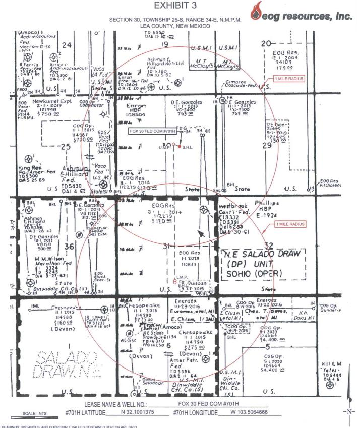
ALL BEARINGS, DISTANCES, AND COORDINATE VALUES CONTAINED HEREON ARE GRID BASED UPON THE NEW MEXICO STATE PLANE COORDINATE SYSTEM, EAST ZONE OF THE NORTH AMERICAN DATUM 1927, U.S. SURVEY FEET
