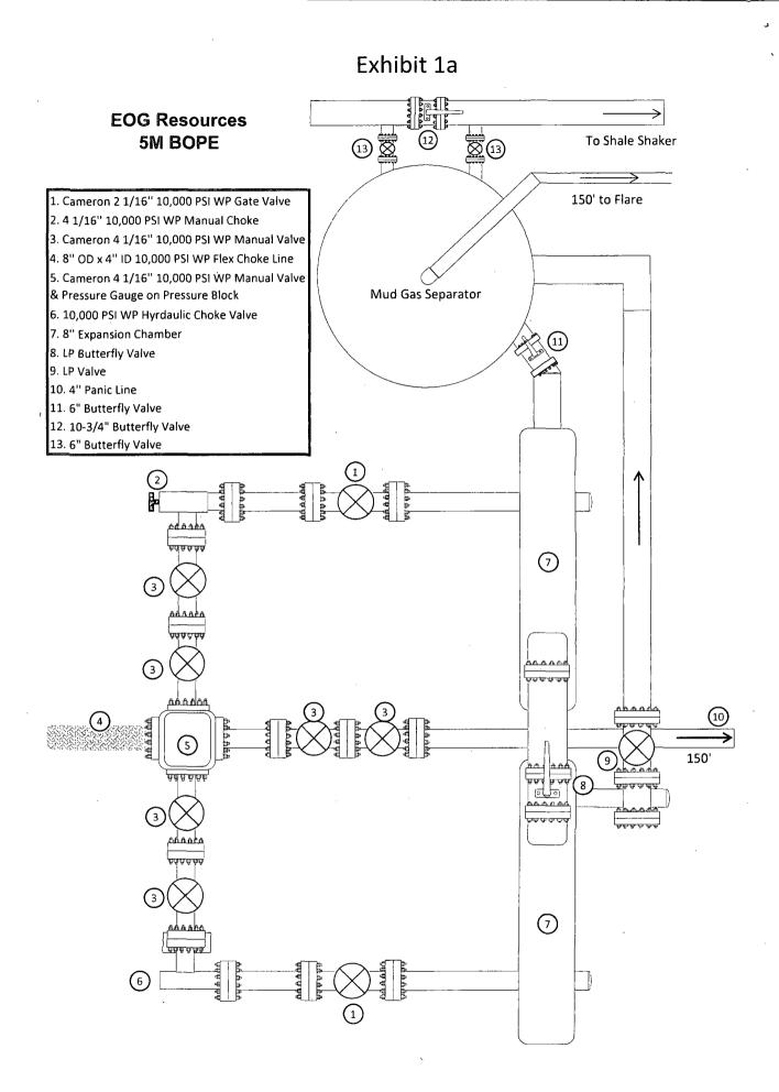
EOG 5M Choke Manifold Diagram (rev. 3/21/14)
