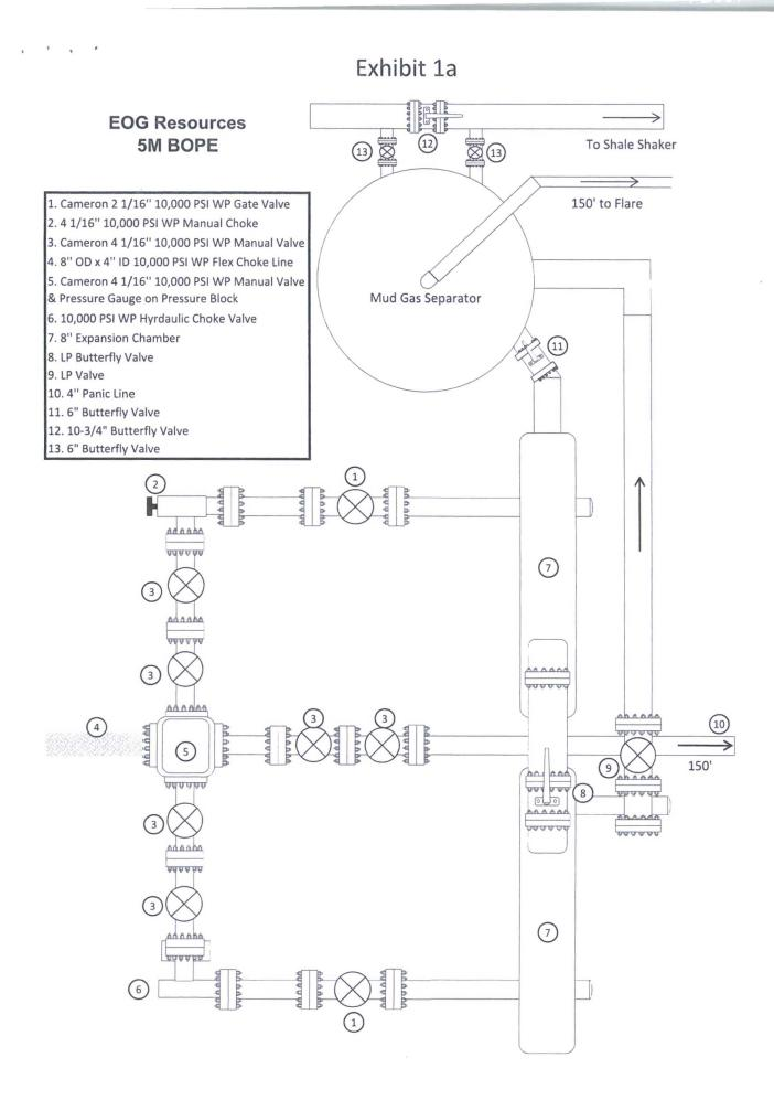
EOG 5M Choke Manifold Diagram (rev. 3/21/14)
