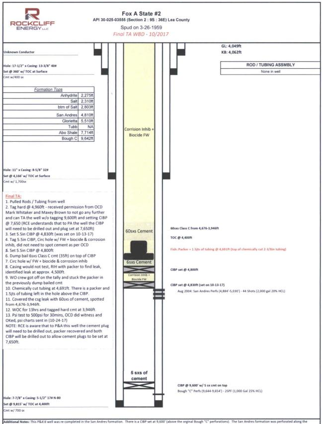
Additional Notes: This P&A'd well was re-completed in the San Andres formation. There is a CIBP set at 9,600' (above the orginal Bough "C" perforations). The San Andres formation was perforated along the interval 4,884-5,030' and tubing was set at 5,030'.
