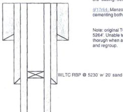
$\frac{\text{History}_1}{4/17/64}. \text{Well abandoned by Jake L. Hamon; recovered 9000' of 7" casing and 1422 of 9-5/8" casing. Set cement plugs up to surface and set 4" marker.}$
