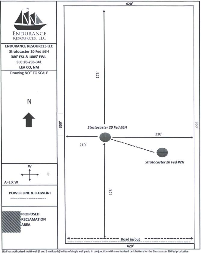
BLM has authorized multi-well (2 and 3 well pads) in lieu of single well pads, in conjunction with a centralized tank battery for the Stratocaster 20 Fed productive wells. No reclamation is proposed at this time. Tank battery and wellsite will be constructed as needed by operations.
