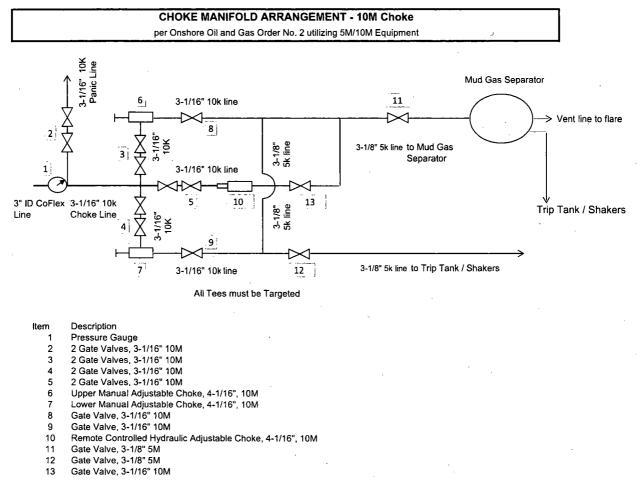
The 10M Choke Manifold & Valves will be tested to rated working pressure.
