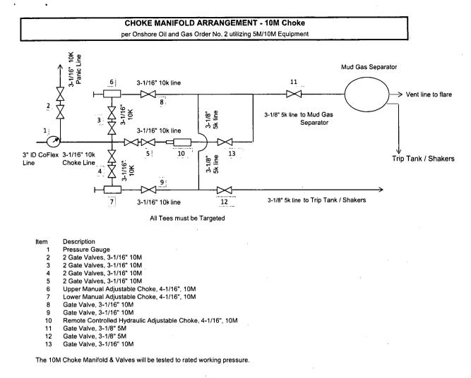
\*Choke manifold will have one remotely operated valve and a manual adjustable valve in front of the choke manifold, as detailed in the Onshore Order 2. It currently contains one 10M hydraulic choke for a total of three choke branches (two manual and one hydraulic).
