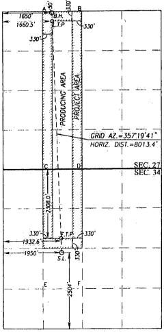
BOTTOM HOLE LOCATION BOTTOM HOLE LOCATION NAD 27 NME NAD 83 NME Y= 404055.9 N Y= 404113.6 N X= 738522.8 E X= 779709.1 E LAT.=32.108523° N LAT.=32.108648' N LONG. = 103.562993° W LONG.=103.563464° W LAST TAKE POINT LAST TAKE POINT NAD 27 NME NAD 83 NME Y= 403776.0 N Y= 403833.8 N X= 779722.2 E X= 738535.9 E LAT.=32.107753° N LAT.=32.107878' N LONG.=103.563428' W LONG. = 103.562957° W
