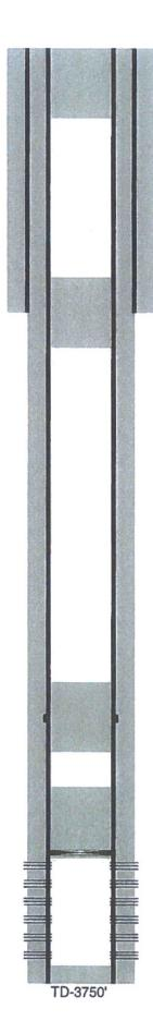
12-1/4" hole @ 1066' 8-5/8" csg @ 1066' w/ 1080sx-TOC-Surf-Circ
