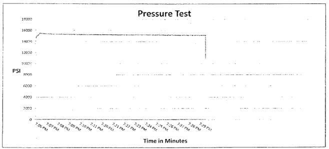
Test Pressure 15000 PSI Time Held at Test Pressure 15 2/4 Minutes
