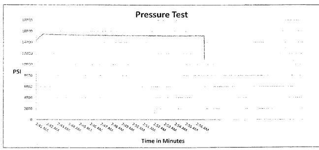
Test Pressure 15000 PSi Time Held at Test Pressure 15 2/4 Minutes Actual Burst Pressure
