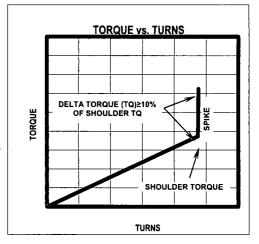
When using Torque vs. Turn monitoring equipment, GB recommends setting a reference torque value of 500 ft.-lbs. or 10% of the minimum makeup torque (whichever is lower) to normalize the resulting plots. Plot scales should be set so data spans at least 2/3 of the turns scale on each plot (10 turns will usually be sufficient at the start and can be reduced based on data from the first few joints). UNDER NO CIRCUMSTANCE SHOULD MAKEUP BE STARTED UNTIL THE MONITORING SYSTEM IS READY TO RECORD DATA.
