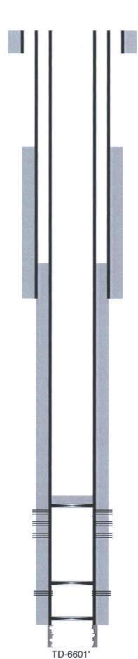
17-1/2" hole @ 301' 13-3/8" csg @ 301' w/ 300sx-TOC-Surf-Circ
