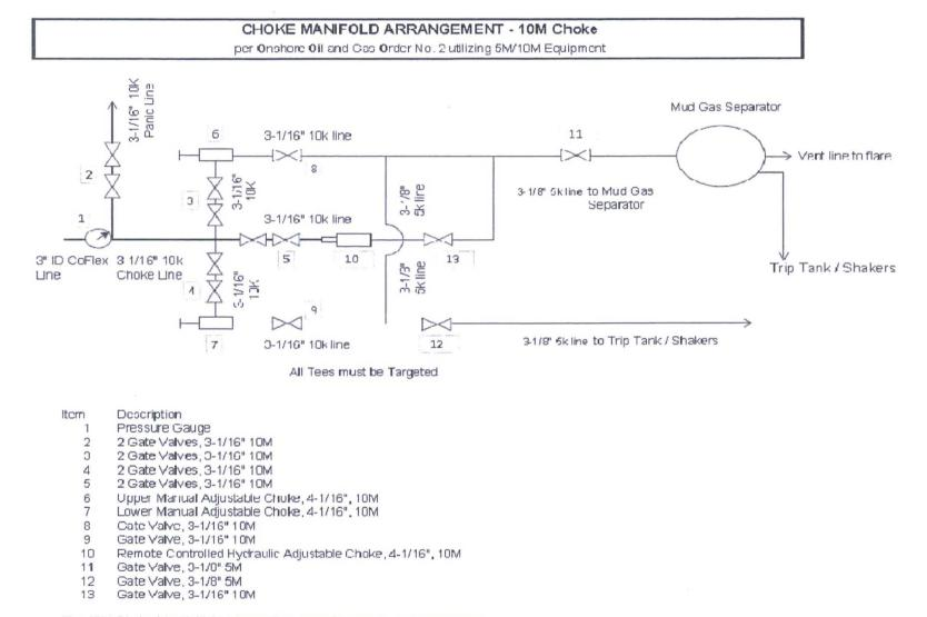
The 10M Choke Manifold & Valves will be tested to rated working pressure.
