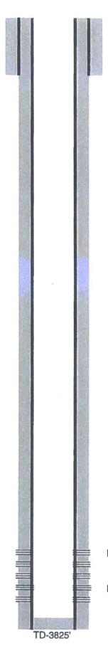
12-1/4" hole @ 396' 8-5/8" csg @ 394' w/ 260sx-TOC-Surf-Circ
