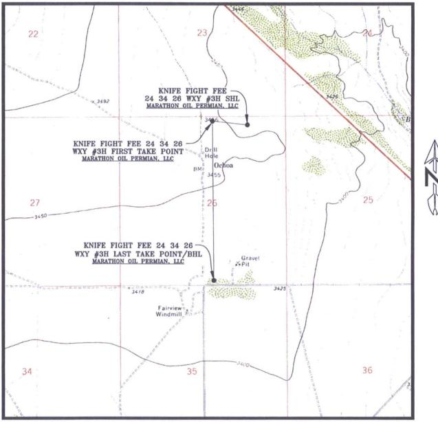
SEC. 26 TWP. 24-S RGE. 34-E SURVEY: N.M.P.M. COUNTY: LEA DESCRIPTION: 271' FNL & 1205' FEL ELEVATION: 3447' OPERATOR: MARATHON OIL PERMIAN, LLC LEASE: KNIFE FIGHT FEE 24 34 26 U.S.G.S. TOPOGRAPHIC MAP: WOODLEY FLAT, N.M. SCALE: 1" = 2000' CONTOUR INTERVAL = 20'
