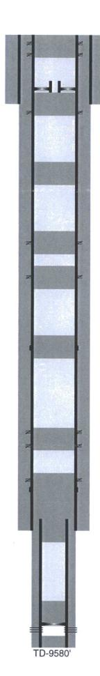
Perf @ 60' Perf @ 250' 17-1/2" hole @ 1110' 13-3/8" csg @ 1110' w/ 1200sx-TOC-Surf-Circ
