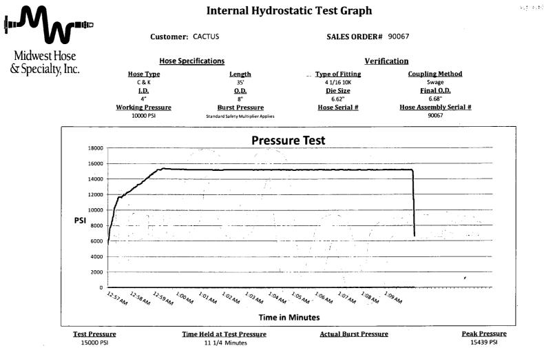
Comments: Hose assembly pressure tested with water at ambient temperature.
