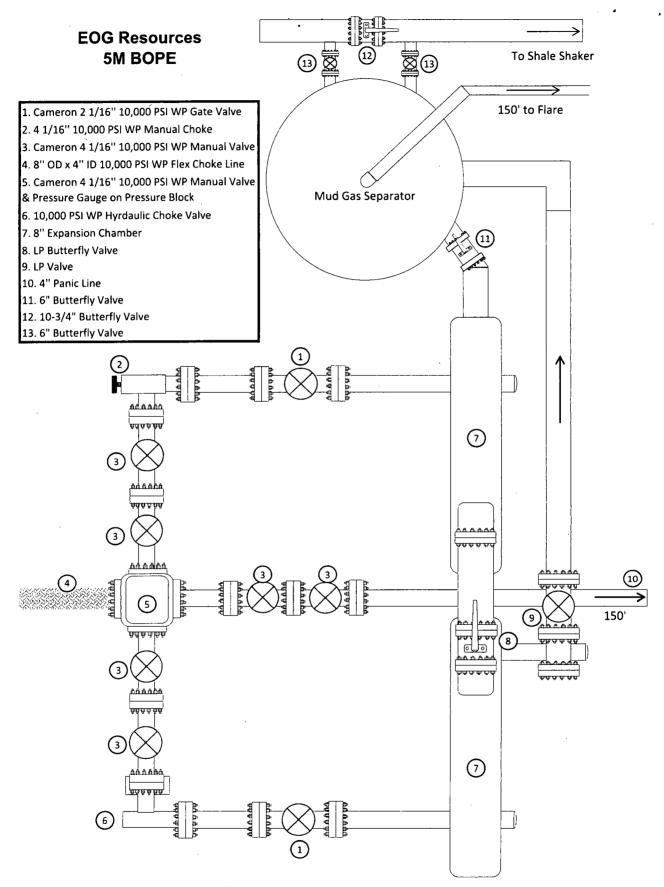
EOG 5M Choke Manifold Diagram (rev. 3/21/14)
