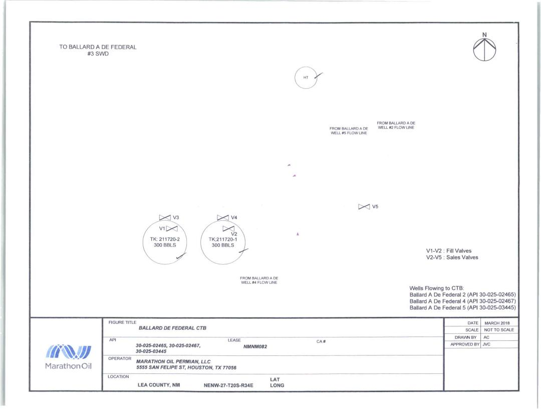
Valve Positioning in the Production Phase
