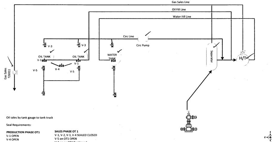
V-1 OPEN V-4 OPEN V-5 SEALED CLOSED Valves on OT2: V-1 CLOSED V-2 CLOSED OR OPEN V-3 SEALED V-5 SEALED CLOSED
