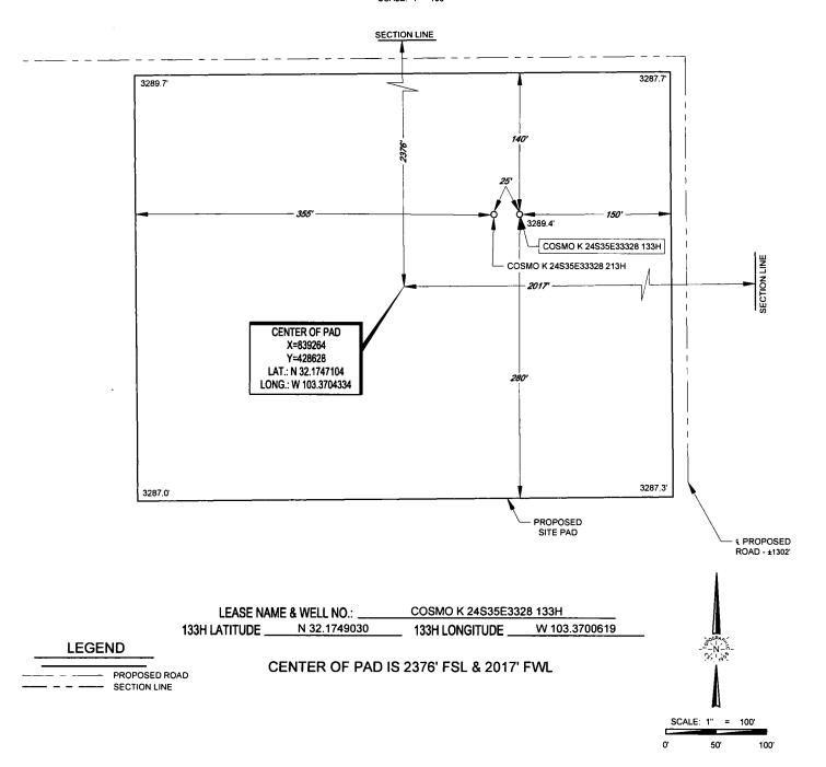
ALL BEARINGS, DISTANCES, AND COORDINATE VALUES CONTAINED HEREON ARE GRID BASED UPON THE NEW MEXICO COORDINATE SYSTEM OF 1983, EAST ZONE, U.S. SURVEY EET.
