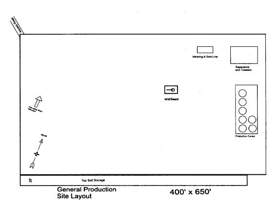
Planned equipment – 2-1000 bbl water tanks and 5-1000 bbl oil tanks, a temporary 6X20 horizontal 3-phase sep., a 48" x 10' 3-phase sep., a 8 X 20' heater treater and a 48" X 10' 2-phase sep.
