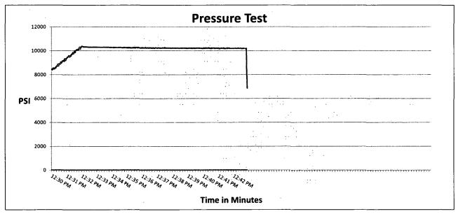
Test Pressure 10000 PSI <u>Time Held at Test Pressure</u> 11 2/4 Minutes **Actual Burst Pressure**
