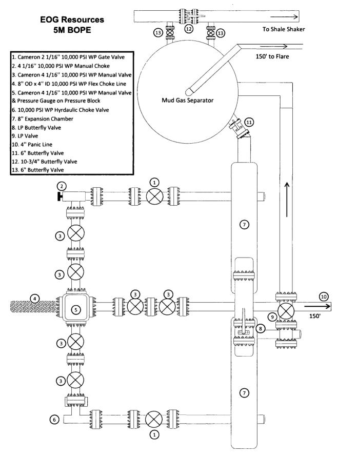
EOG 5M Choke Manifold Diagram (rev. 3/21/14)
