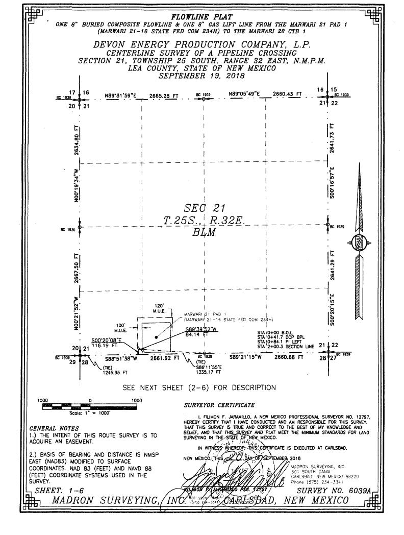
FLOWLINE PLAT ONE 8" BURIED COMPOSITE FLOWLINE & ONE 8" CAS LIFT LINE FROM THE MARWARI 21 PAD 1 (MARWARI 21-16 STATE FED COM 234H) TO THE MARWARI 28 CTB 1 DEVON ENERGY PRODUCTION COMPANY, L.P. CENTERLINE SURVEY OF A PIPELINE CROSSING SECTION 21, TOWNSHIP 25 SOUTH, RANGE 32 EAST, N.M.P.M. LEA COUNTY, STATE OF NEW MEXICO SEPTEMBER 19, 2018 DESCRIPTION
