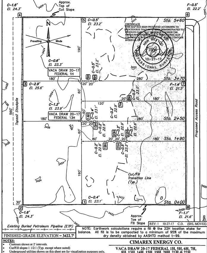
Underground utilities shown on this sheet are for visualization purposes only, actual locations to be determined prior to construction.
