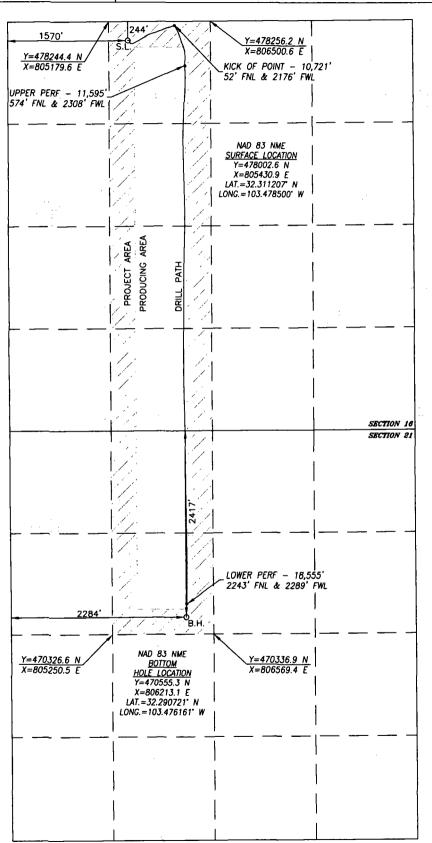
BOREPATH SHOWN HEREON IS BASED ON DIRECTIONAL SURVEY REPORT PROVIDED BY COG OPERATING, LLC FOR THE GETTYSEURG STATE COM \$13H SUPPLIED TO HARCOW SURVEYING, LLC ON NOVEMBER 9, 2018
