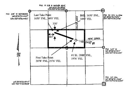
OVES! BASIS OF BEARING IS A TRANSPERSE MERCATOR PROJECTION OF THE NEW MEXICO STATE FLAME COORDINATE SYSTEM, EAST ZONE (3001), IND 83 (CORS86) . SCALE 1" = 2010"
