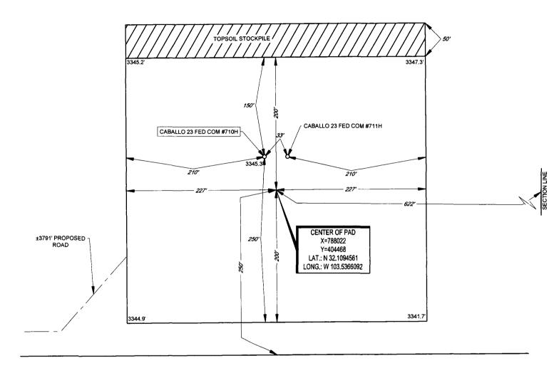
ALL BEARINGS, DISTANCES, AND COORDINATE VALUES CONTAINED HEREON ARE GRID BASED UPON THE NEW MEXICO COORDINATE SYSTEM OF 1983, EAST ZONE, U.S. SURVEY FEET.
