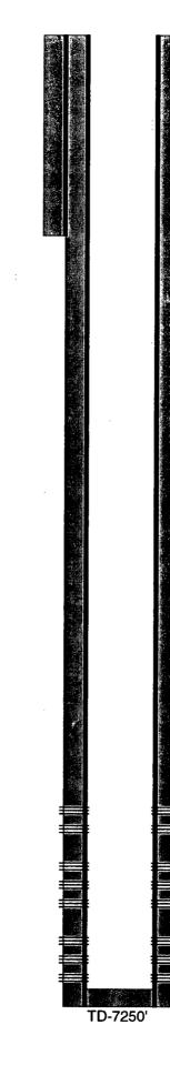
7-7/8" hole @ 7250' 5-1/2" csg @ 7250' w/ 1680sx-TOC-Surf-Circ
