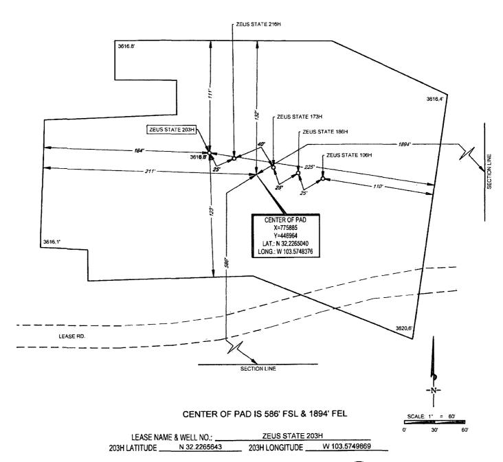
ALL BEARINGS, DISTANCES, AND COORDINATE VALUES CONTAINED HEREON ARE GRIO BASED UPON THE NEW MEXICO COORDINATE SYSTEM OF 1983, EAST ZONE, U.S. SURVEY FEET
