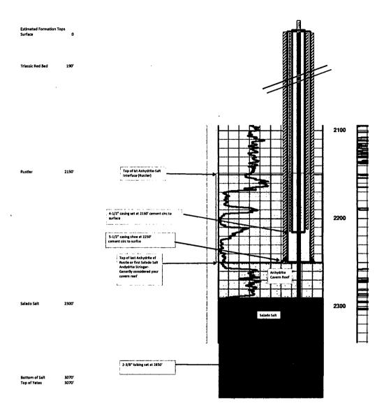
Wasserhund BW-22 Well Bore Skematic and Formation Tops Superimposed on Llano Disposal, LLC st4 #1 API 30-025-26370 2 miles south sec 4-Ts13s-R363. CN-GR Log
