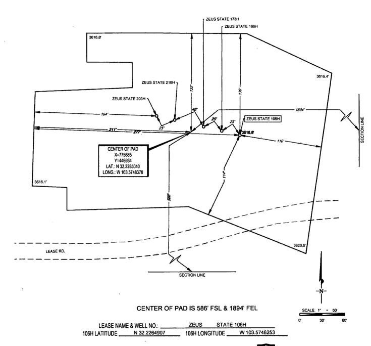
ALL BEARINGS, DISTANCES, AND COORDINATE VALUES CONTAINED HEREON ARE GRID BASED UPON THE NEW MEXICO COORDINATE SYSTEM OF 1983, EAST ZONE, U,S, SURVEY FEET
