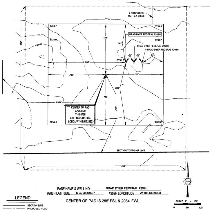
ALL BEARINGS, DISTANCES, AND COORDINATE VALUES CONTAINED HEREON ARE GRID BASED UPON THE NEW MEXICO COORDINATE SYSTEM OF 1983, EAST ZONE, U.S. SURVEY FEET
