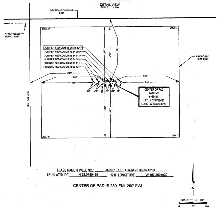
ALL BEARINGS, DISTANCES, AND COORDINATE VALUES CONTAINED HEREON ARE GRID BASED UPON THE NEW MEXICO STATE PLANE COORDINATE SYSTEM, EAST ZONE OF THE NORTH AMERICAN DATUM 1983, U.S. SURVEY FEET
