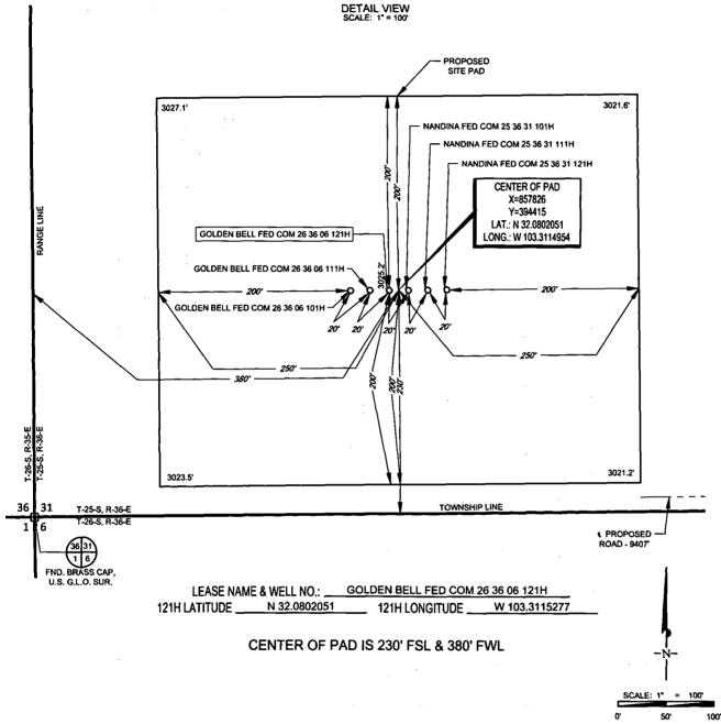
ALL BEARINGS, DISTANCES, AND COORDINATE VALUES CONTAINED HEREON ARE GRID BASED UPON THE NEW MEXICO STATE PLANE COORDINATE SYSTEM, EAST ZONE OF THE NORTH AMERICAN DATUM 1983, U.S. SURVEY FEET
