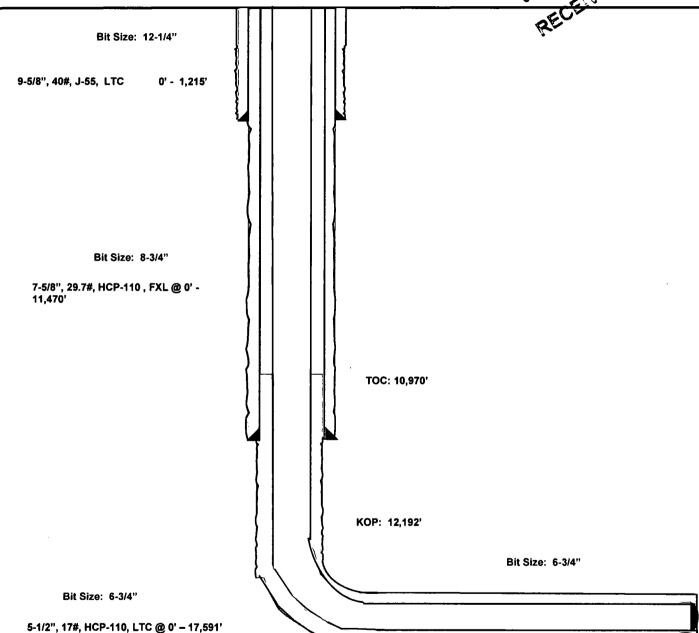
Lateral: 17,591' MD, 12,508' TVD BH Location: 100' FSL & 330' FEL Section 2 T-25-S, R-33-E 388' FNL 1680' FEL Section 2 T-25-S, R-33-E
